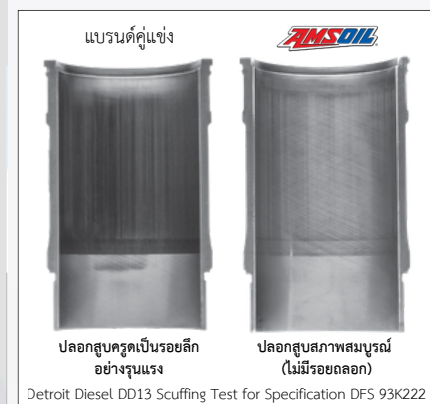
DETROIT DIESEL DD13 SCUFFING TEST FOR SPECIFICATION DFS 93K222
